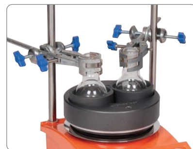
Multi-Well Block accepts small flasks from 10 ml
