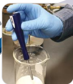
ASAP ® : Atmospheric Solids Analysis Probe
