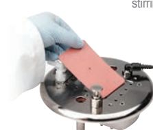
GreenHouse Plus allows additions and withdrawals through sealing mats
