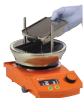
Insert the adapter into the GreenHouse base
