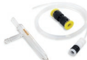
SeaSpray concentric nebulizer (standard on the 5000 series ICP-OES), G8010-60255
