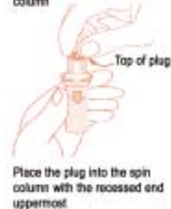
Loading the plug into the spin column
